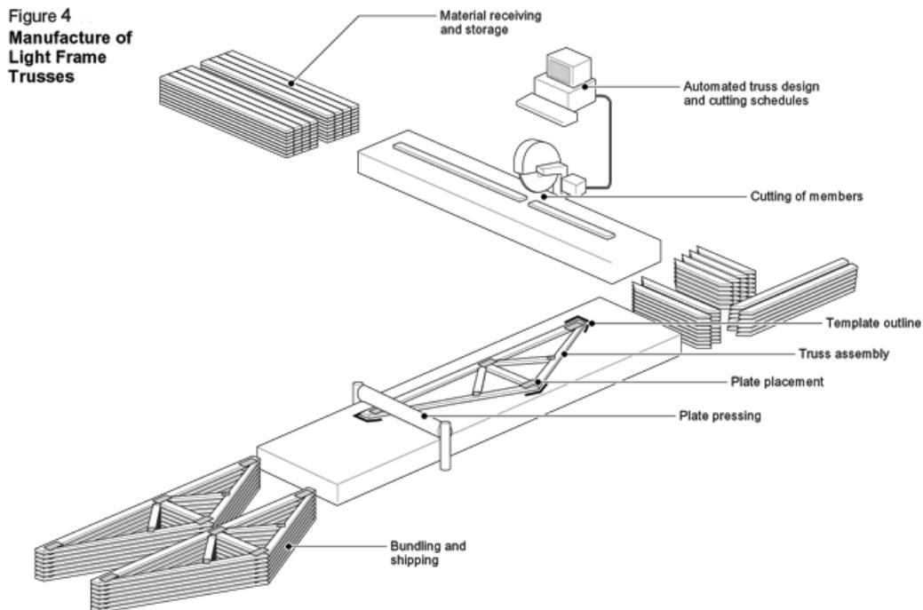
When the pressing of the plates has been completed, the trusses are checked for dimensions, wood to wood gaps, lumber size and species, plate size, positioning and embedment and moved to a storage area. In some cases plants have a quality control program that ensures consistency in production and quality in place of checking each truss. The completed trusses are then strapped together and placed in the storage yard in preparation for shipping.
