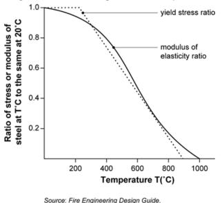
Figure 1: Steel loses strength at elevated temperatures
