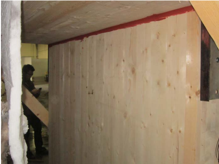
Exposed Side before the Fire Test
