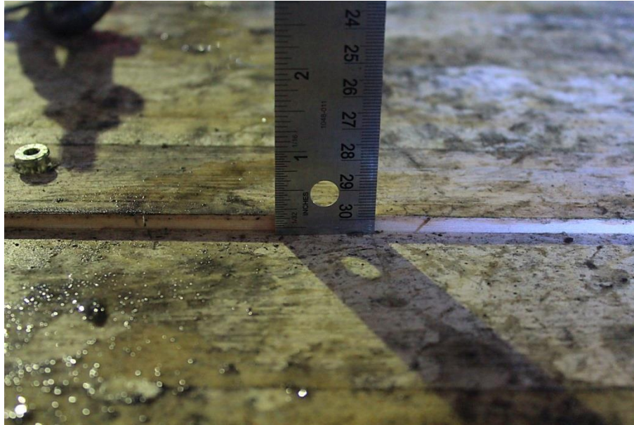
Figure 18. Differential deflection of the 7-ply half-lapped joint
