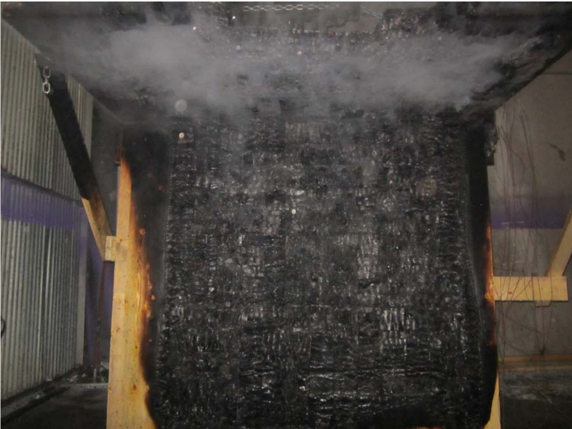
Exposed Side After Fire Test
