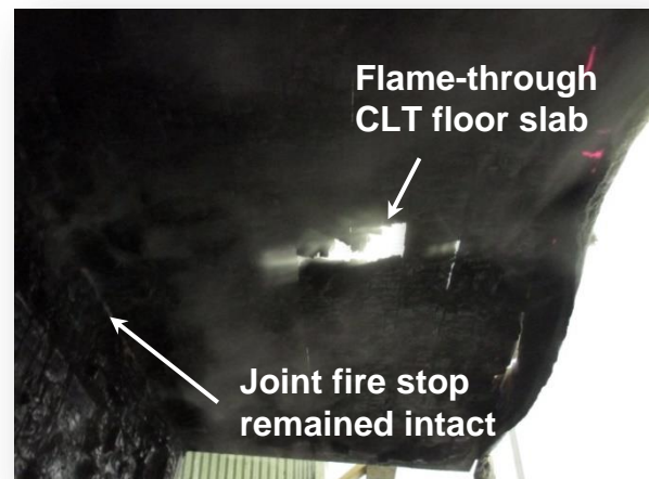
Figure 11. Visual observations from test sample No.3
