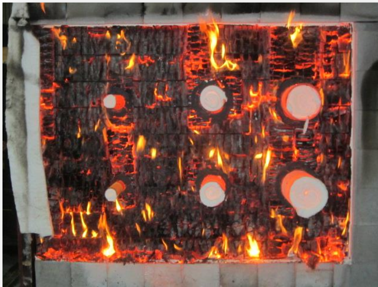
Figure 15. Test sample No.6 removed from furnace
