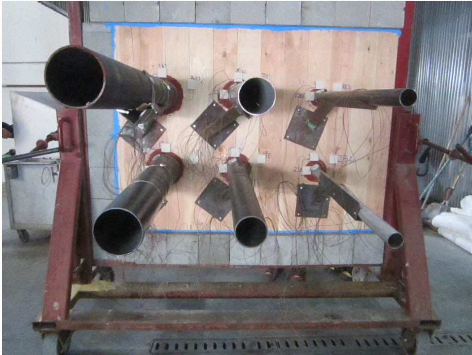
Unexposed Side Prior to the Fire Test
