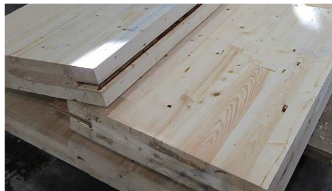
b) Internal spline
