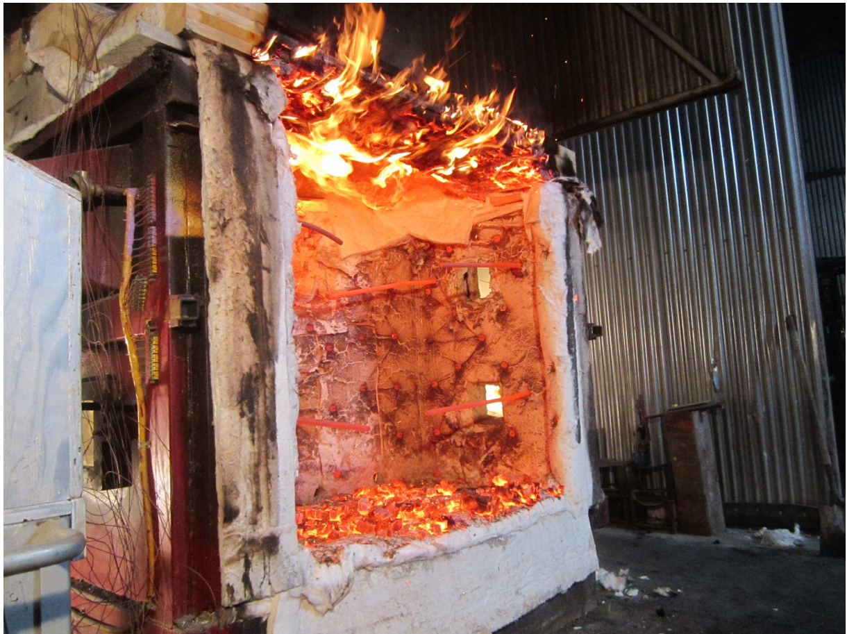
Exposed Side After the Fire Test
