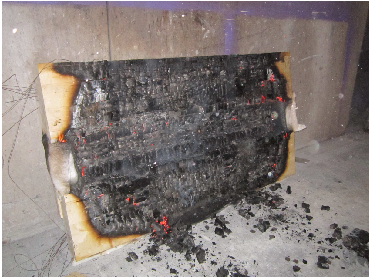
Exposed Side After the Fire Test
