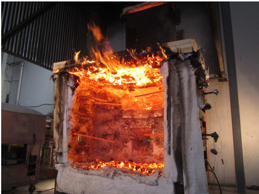
Exposed Side After the Fire Test
