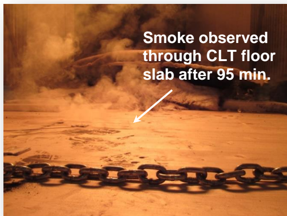
Figure 11. Visual observations from test sample No.3
