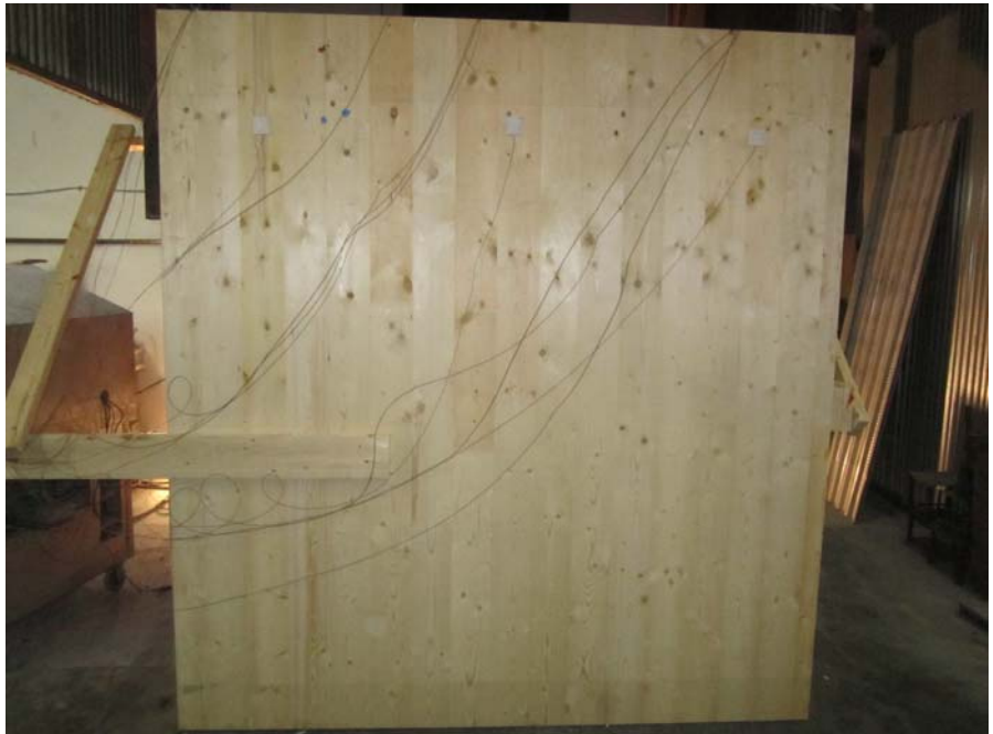
Unexposed Side Prior to the Fire Test
