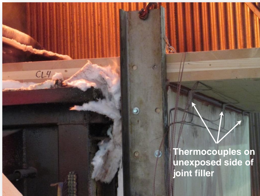
Figure 4. Thermocouple locations for linear joint No. 3 (Wall-to-Floor)
