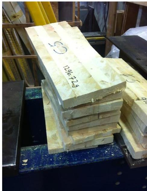
Figure 6. Transversalslices for Series C used for Moisture Content and Specific Gravity
