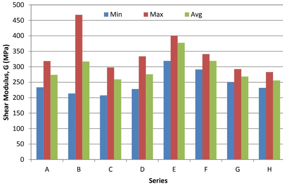
Figure 7. Minimum, Maximum, and Average Shear Moduli
