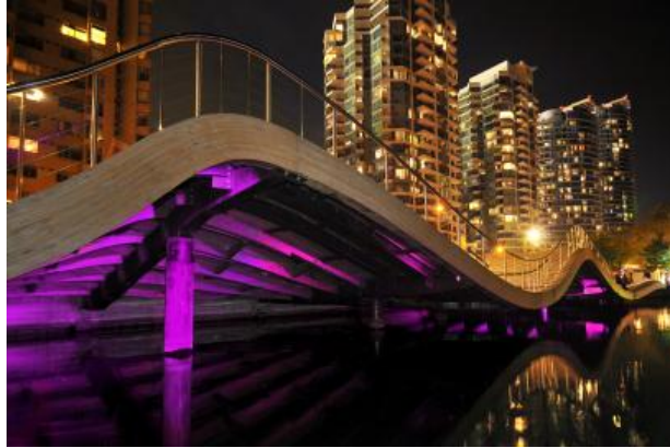
Figure 19. Wavedeck in Toronto using yellow cedar glulam
