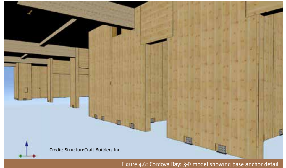
Figure 4.6: Cordova Bay: 3-D model showing base anchor detail
