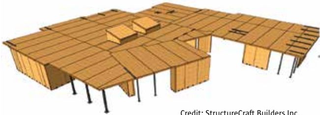
Figure 4.4: Cordova Bay: 3-D model of wood structure
