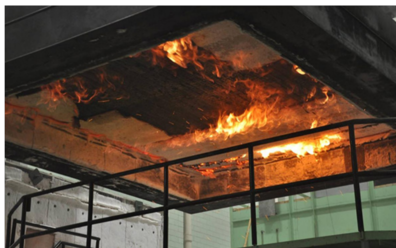
Figure 3.4. Photo taken at the end of a fire-resistance test on a 3-ply CLT floor assembly protected with gypsum board.
