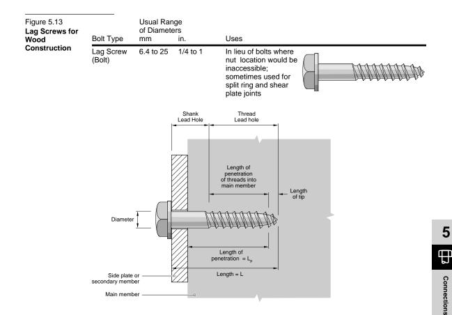
The resistance of a lag screw generally increases with the length of the embedded threaded portion. However, it is also affected by other considerations such as side plate thickness.
