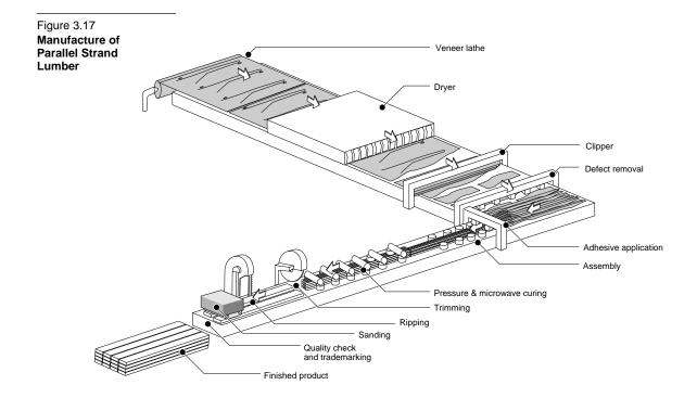
The billet is cross cut to desired lengths, rip sawn to produce rough stock dimensions or custom sizes, and sanded down to finish dimensions. Larger dimensions are produced by edge gluing billets together using techniques common to those used for the manufacture of glulam.
