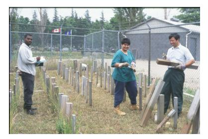
Testing of treated lumber and sawn posts at the northerly limit of termite activity in Ontario. This test site is maintained in collaboration with the City of Kincardine. Termites eat through a thin shell of preservative treatment, but material meeting the penetration requirements of CSA standards performs well.
