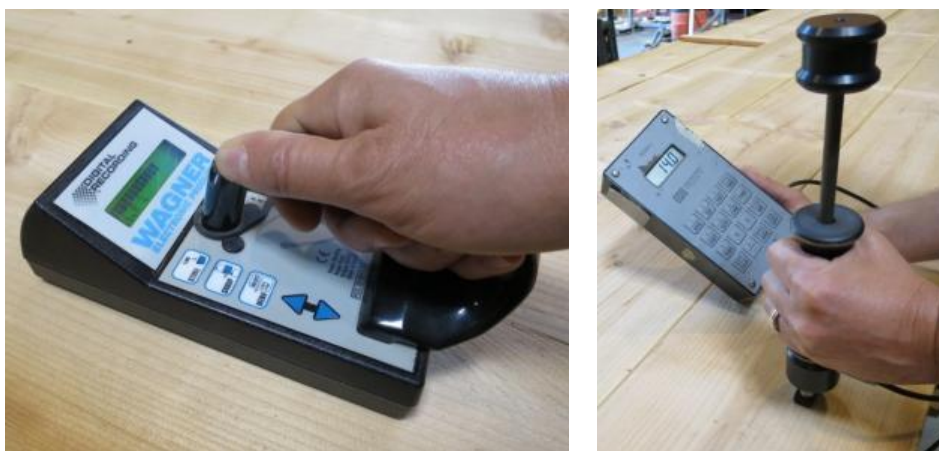
Figure 6 Measuring wood moisture content using a capacitance-based meter (left) and a resistance-based meter (right)
