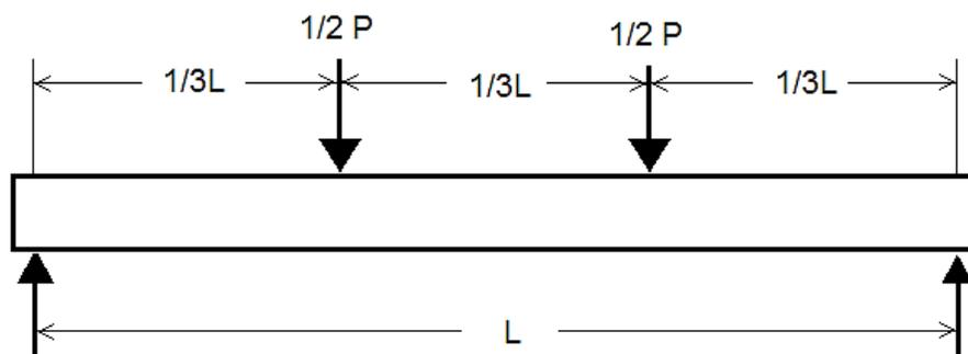
Figure 2. Schematic of the third-point loading setup
