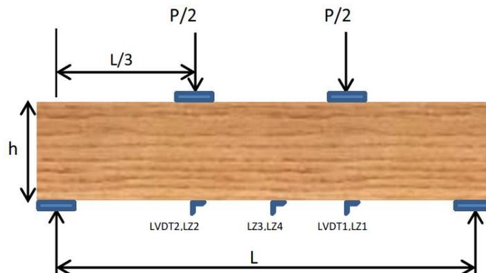
Figure 7. Loading pattern and instrumentation for the 4 feet x 28 feet specimens (Series C)
