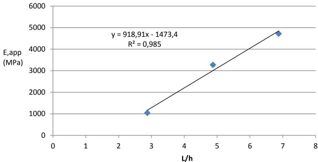
Figure 9. The relationship between the apparent Modulus of Elasticity ( $E_{app}$ ) and the span to depth ratio ( $L/h$ ) for all specimens tested
