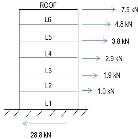
Figure 7. Vertical distribution of seismic forces (Iteration #1)
