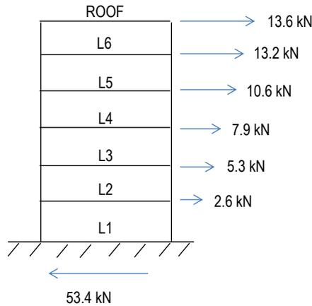
Figure 5. Initial design forces for Wall 1.
