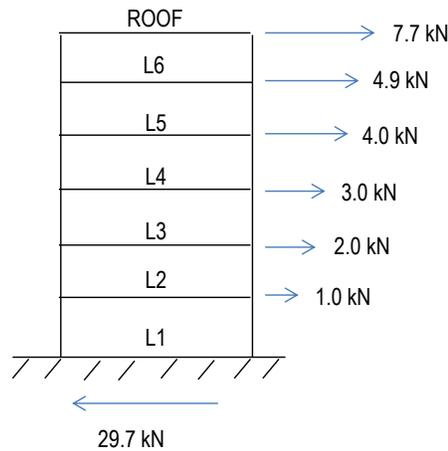
Figure 8. Vertical distribution of seismic forces (Iteration #2)
