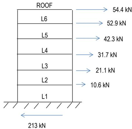
Figure 2. Initial vertical distribution of seismic forces
