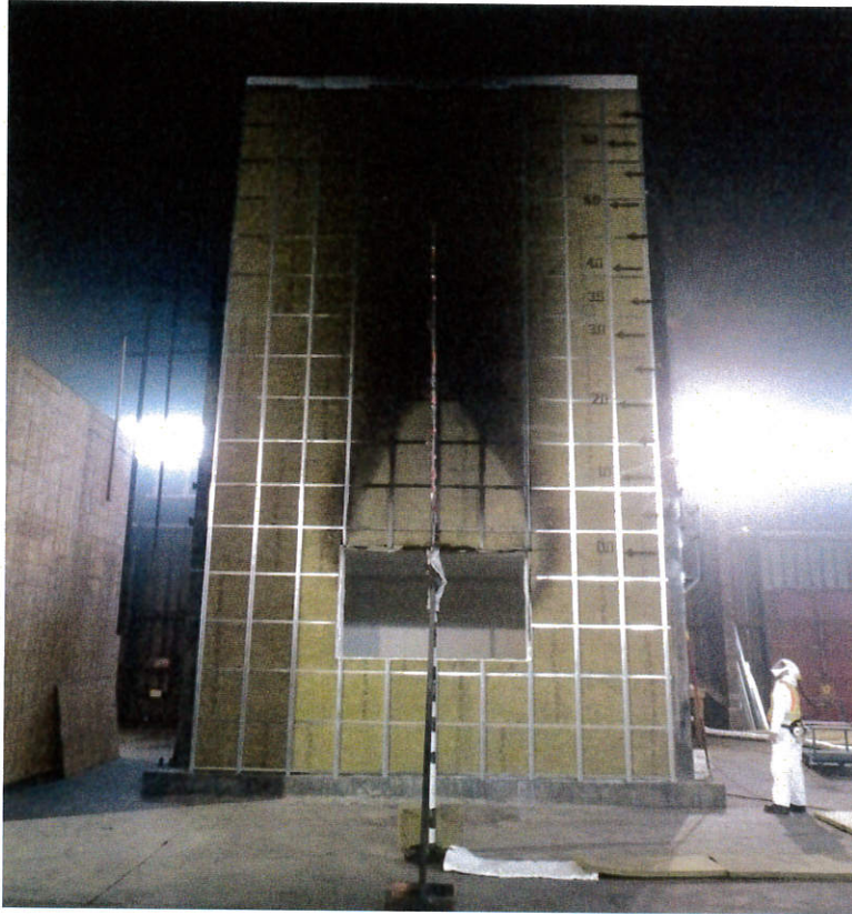
Figure 17. Wall sample after fire exposure.
