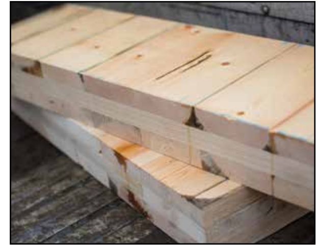
Fig. 4.3: Three-ply CLT panels prior to installation
