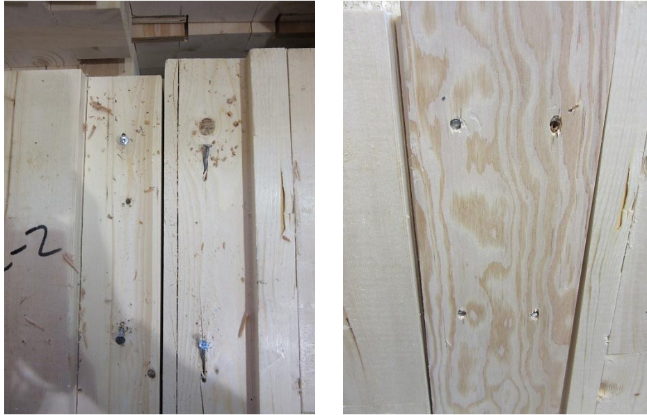
Figure 7. Typical mode of failure for specimens of Series C
