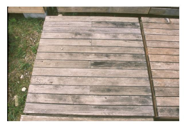
The CCA-treated boards in our decking test are not re-finished with stains or water-repellants which would further improve their appearance and service life. Of the two species within the hem-fir group, Pacific Silver fir is the more treatable and the more dimensionally stable of the two species.
