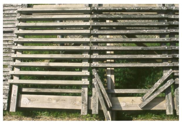
CCA-treated and untreated finger-jointed lumber showing decay at the joints. This is a relatively low decay hazard because the test materials are well-spaced and the test unit does not trap water.
