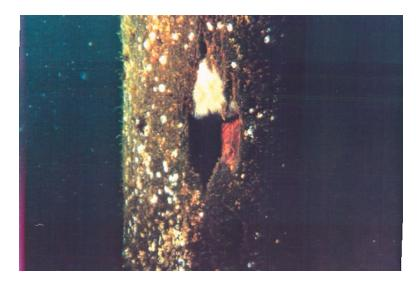
This test of marine piling was originally set up by the Pacific Biological Station, Nanaimo, BC. It was taken over by Forintek and inspected by Foreshore Technologies, funded by Public Works Canada. CCA is not normally recommended for Douglas fir piling. The pile illustrated here was from a separate batch of poorly treated material and is showing severe attack by shipworm.
