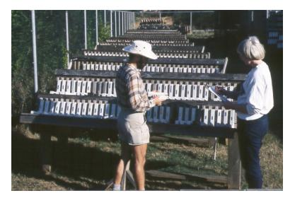
Millwork preservatives are evaluated using an accelerated test, which simulates the lower part of the opening light of a window. No protection from weather is provided, and an initial break in the paint film is deliberately applied. Millwork was once commonly treated with Pentachlorophenol but the registration for this use has been withdrawn.
