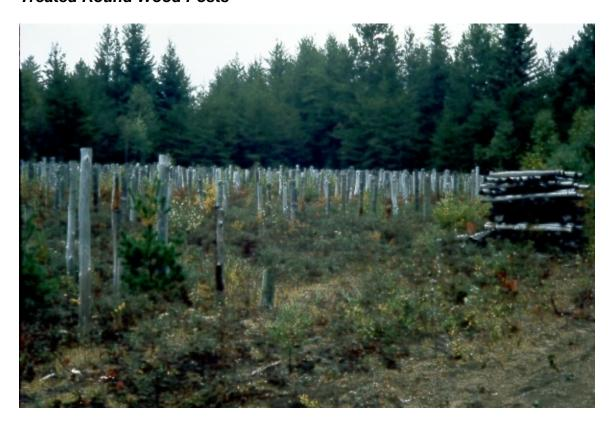
Some of our longest-running tests involve farm-style round fence posts made from forest thinnings. This method can also be used to predict the service life of treated utility poles. In this test, CCA-treated posts have lasted 10 times longer than their untreated counterparts.
