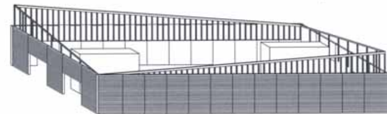
Cementitious board on wood frame construction
