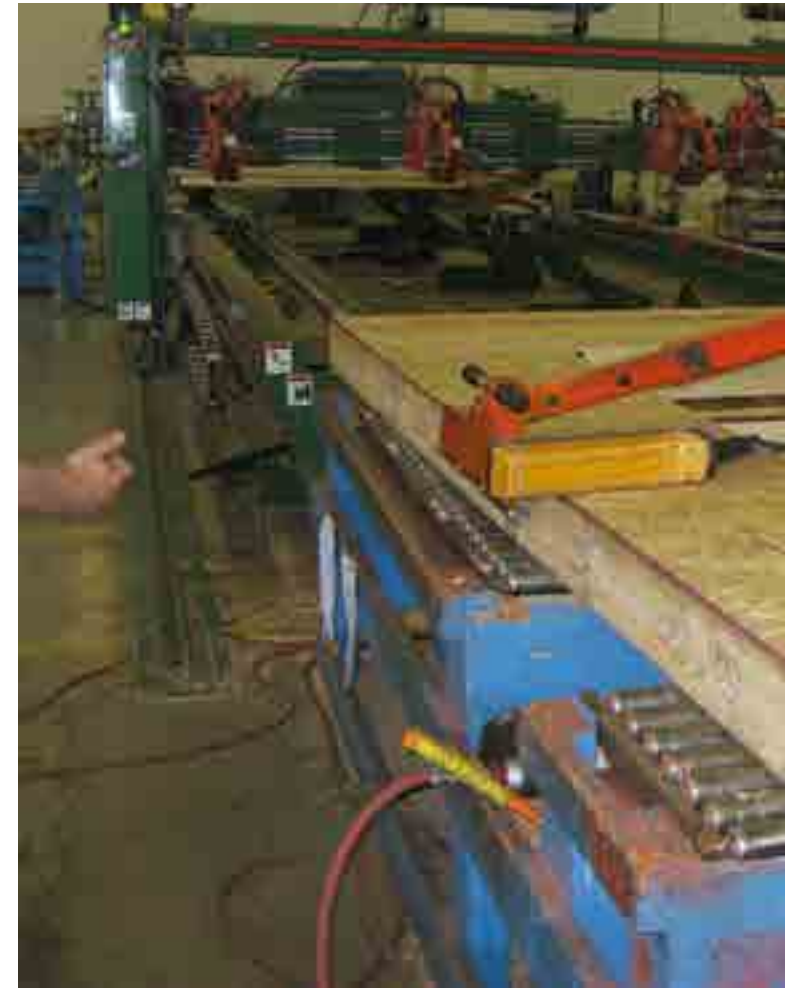
FIGURE 7.1 – HILLCREST VILLAGE: FACTORY PREFABRICATION OF WOOD-FRAME WALLS
