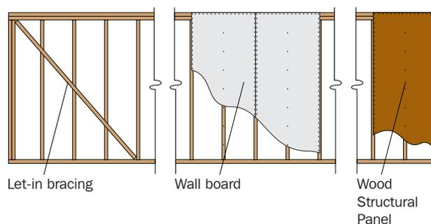
**Engineered Shear Walls**
