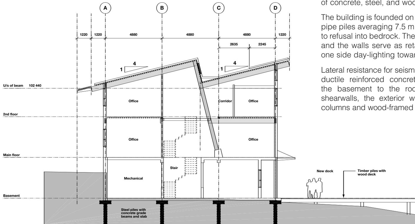
**FIGURE 3** Building Cross-Section
