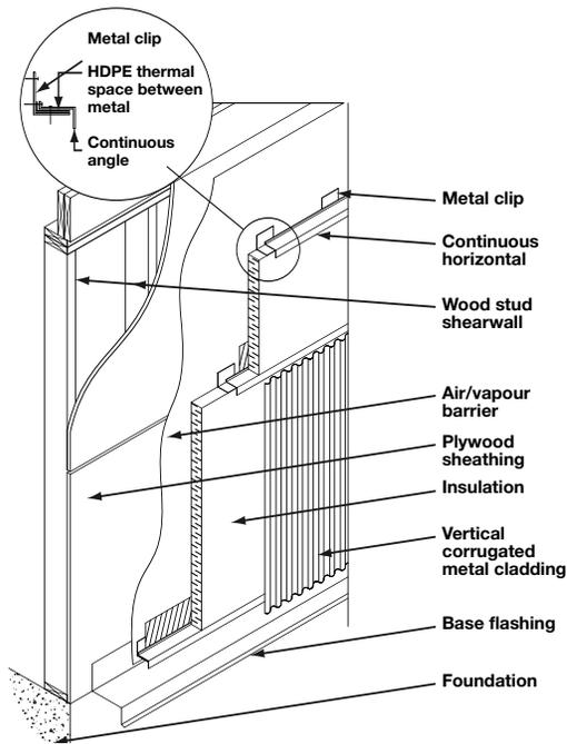
**FIGURE 6** Typical Exterior Wall
