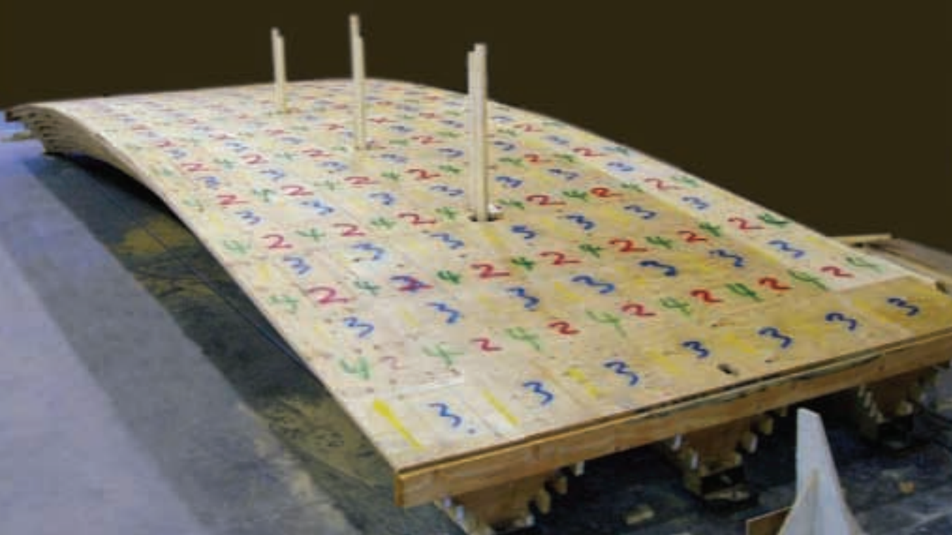
Test panel prior to loading with differential loads
