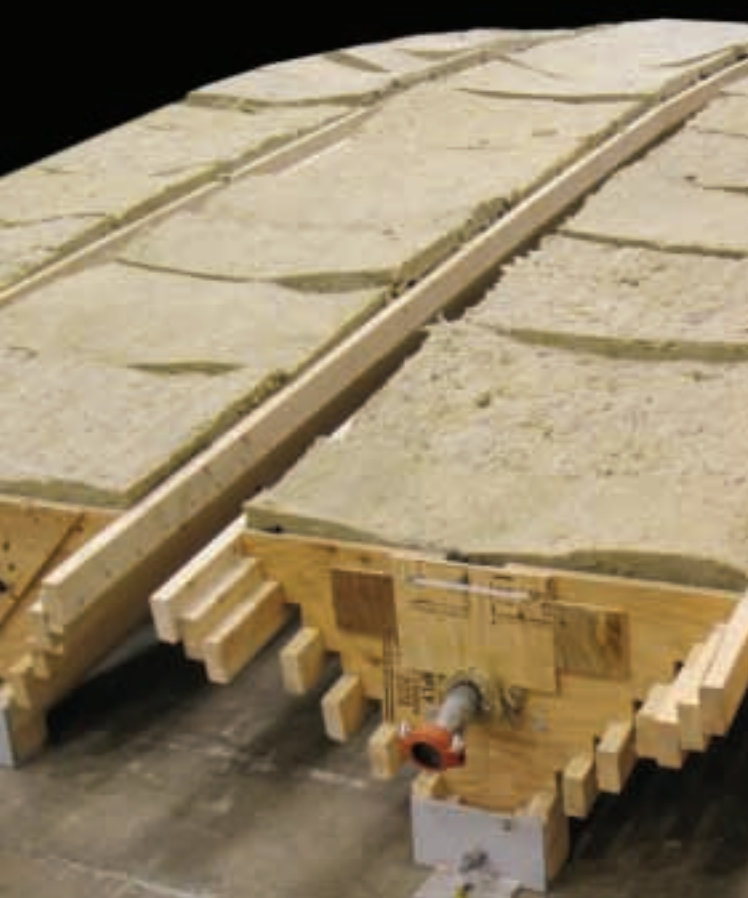
Panel Vees loaded with fibrous insulation
