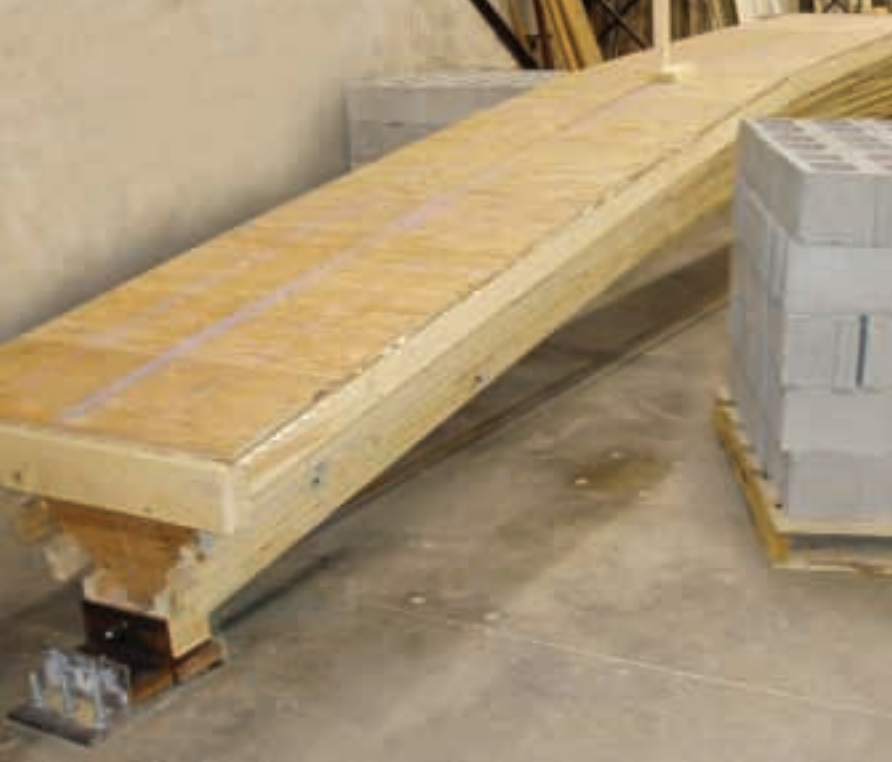
Panel Vee and concrete blocks prior to test loading
