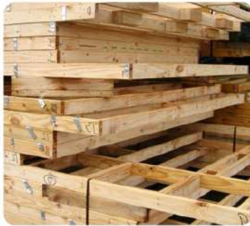
Figure 10: Prefabricated wall frames and floor cassette
