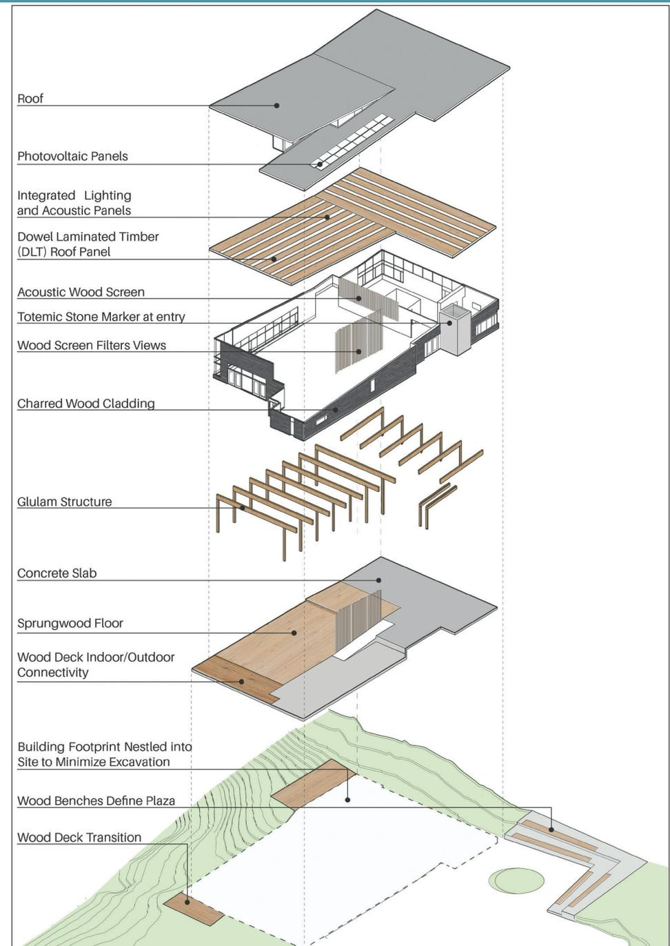
3.9 Exploded view of the structural system, designed by structural engineer Robert Malczyk to accommodate different beam and panel products.
