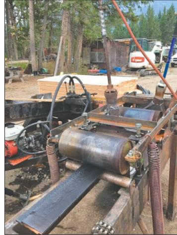
3.6 The siding was charred by running it through a custom machine fitted with propane burners.
