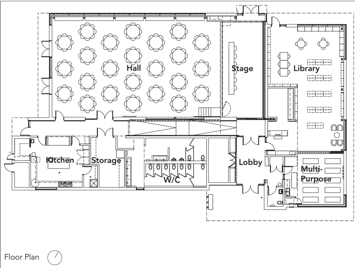
3.3 The plan is arranged along an east-west axis to optimize passive energy performance.
