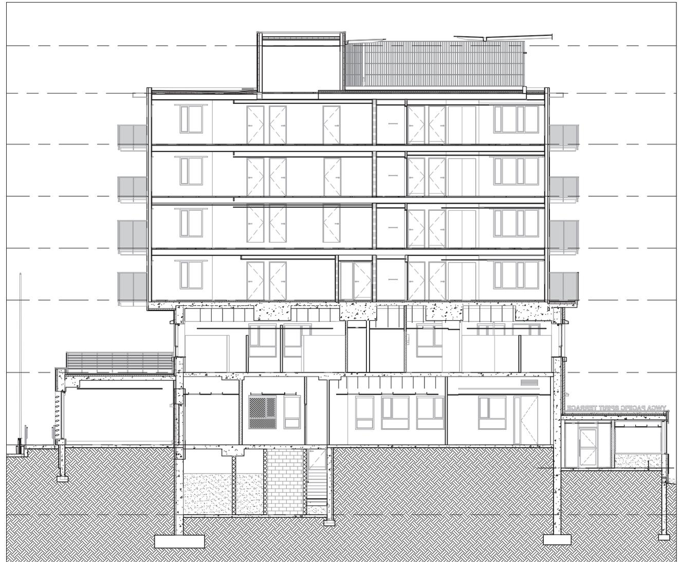
2.8 North-South section: With the overall height limited by the zoning, it was necessary to minimize the structural depth of each floor.
