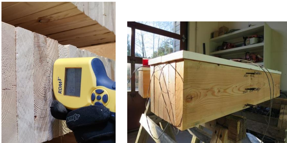
Figure 4 Measuring wood moisture content using a portable pin meter (left) and pre-installed moisture pins (right).
