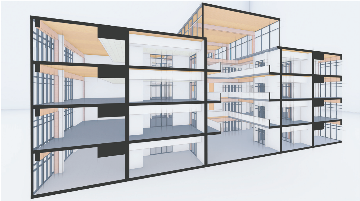
Sectional View Illustrating the Reduction of Interior Finishes for Flat Panel Mass Timber Framing Systems
