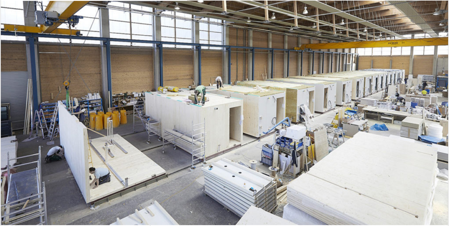
FIG 2: Kaufmann Bausysteme's 3D module production.
