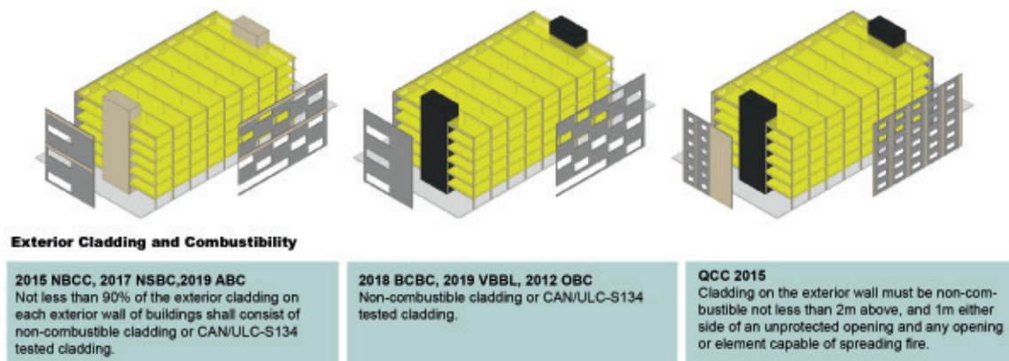
Figure 2.34: Exterior cladding requirements where the exterior cladding is required to be non-combustible except for a limited amount as described above for buildings of 5 to 6 stories in height. Note that buildings of four-storeys or lower may have different requirements depending on the jurisdiction.
