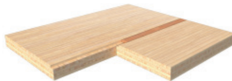
Figure 3.11: Typical CLT spline connection.
