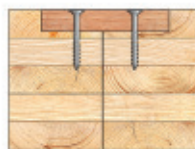
Figure 3.11: Typical CLT spline connection.
