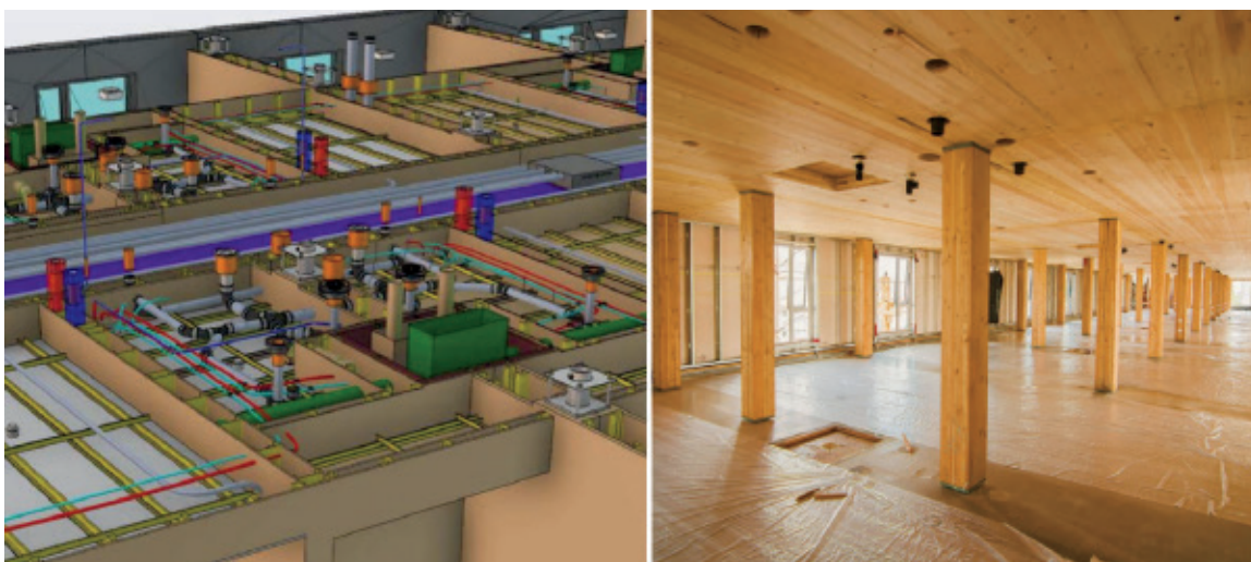
Figure 2.12: Right: Image by Cadmakers illustrating the level of detail involved in coordinating MEPF systems for fabrication. Left: Image of plumbing shelving and penetrations through CLT slab.
