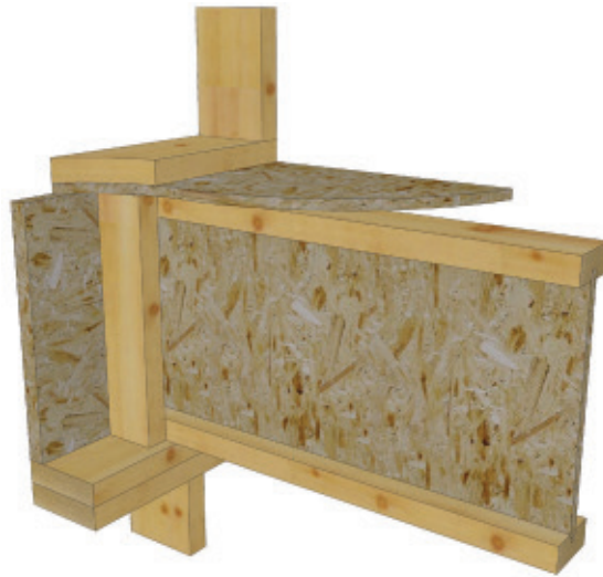
Figure 3.23: Squash block with rim board detail.
