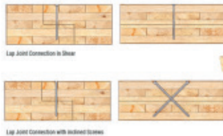
Figure 3.10: Typical CLT lap joint connection.
