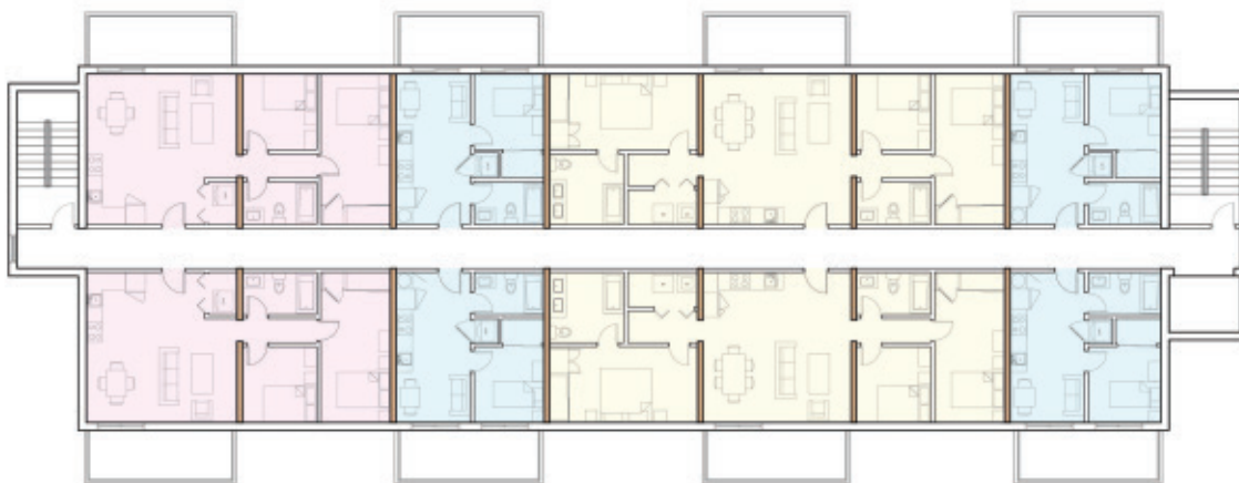
Figure 2.83: Concept floor plan of a CLT multi-storey residential building illustrating a flexible unit design using a modular approach. The plan accommodates one-, two- and three-bedroom suite layouts with consideration of adaptability over time.
