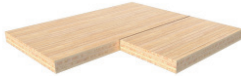
Figure 3.09: Typical CLT butt joint connection.
