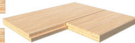
Figure 3.10: Typical CLT lap joint connection.
