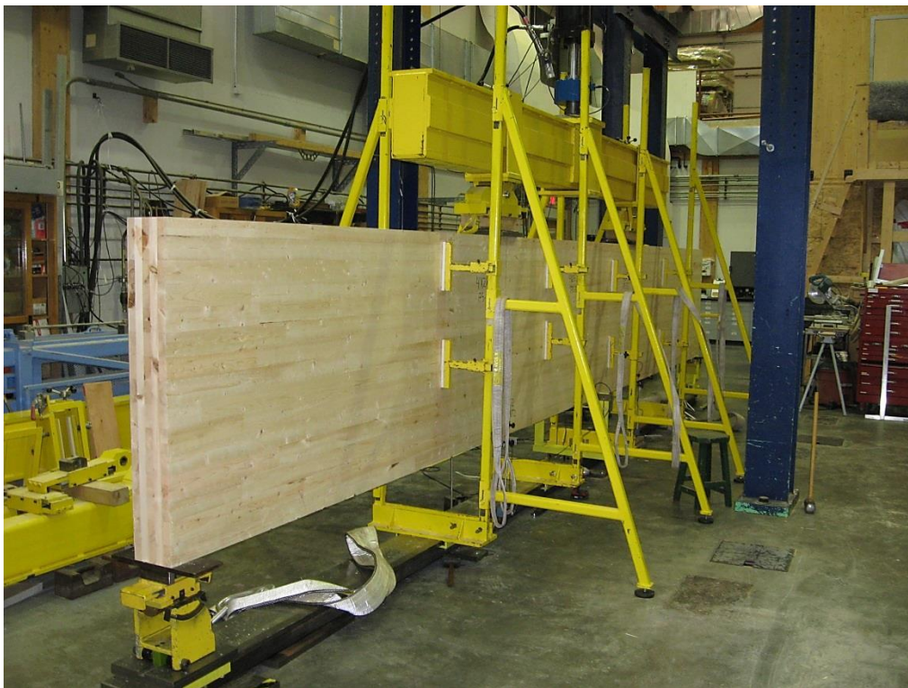
Figure 4. Photo of a specimen from Series C (4 feet x 28 feet) ready for testing
