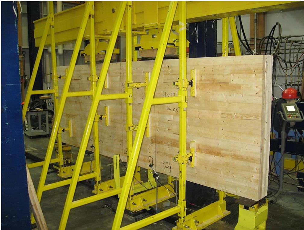
Figure 3. Photo of a specimen from Series A (4 feet x 12 feet) ready for testing
