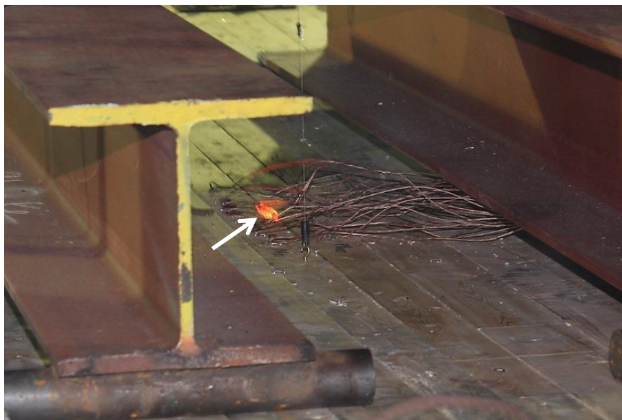
Figure 25. Failure of the 5-ply internal spline
