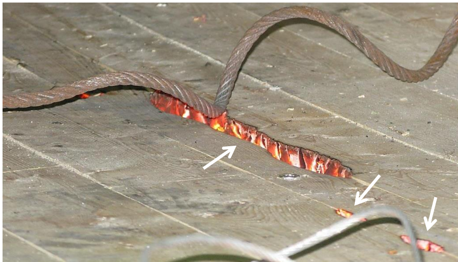
Figure 7. Failure of the 3-ply half-lapped joint
