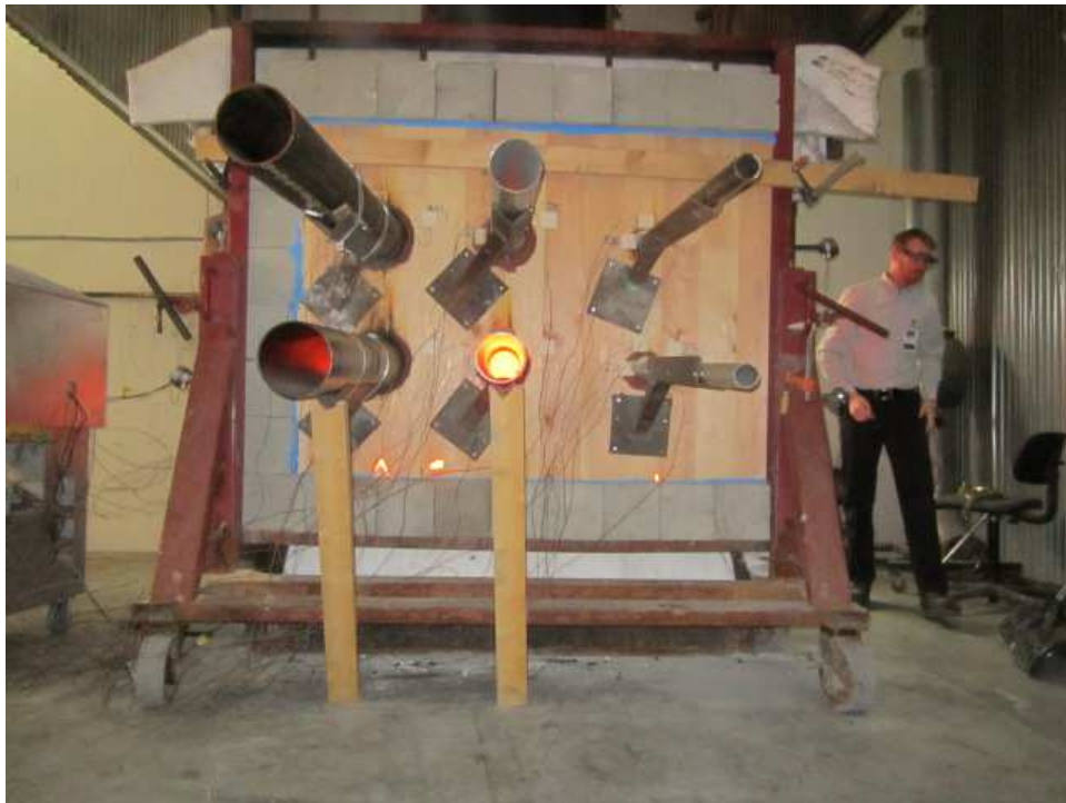
Unexposed Side During the Fire Test
