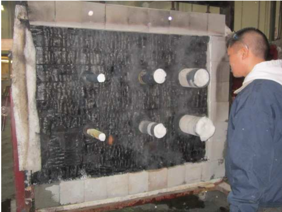
Exposed Side After the Hose Stream Test
