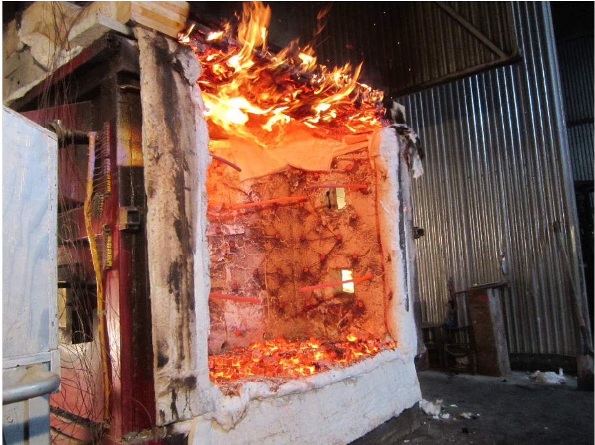
Exposed Side After the Fire Test
