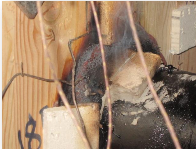
Figure 14. Unexposed surface of the 4 in. cast iron pipe during the test
