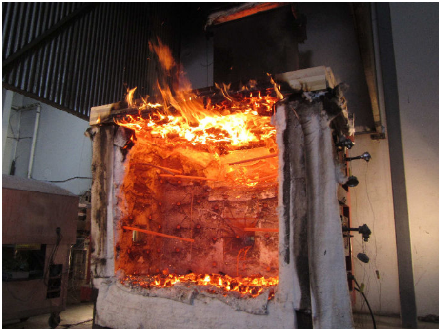
Exposed Side After the Fire Test
