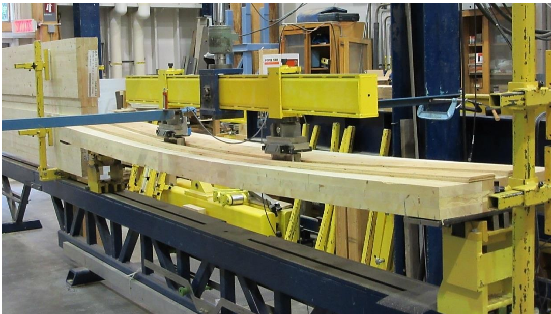
Figure 4. CLT bending test under ambient conditions
