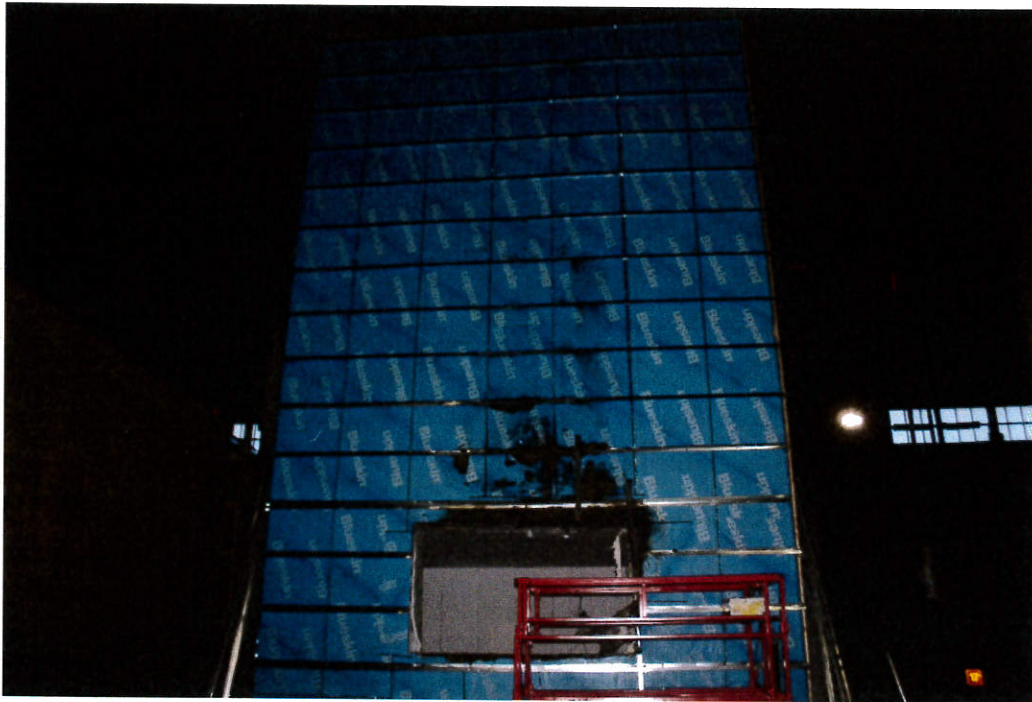
Figure 19. Insulation fully removed (showing water resistant barrier over CLT panels; small pieces of insulation still on the water resistant barrier) after fire exposure.
