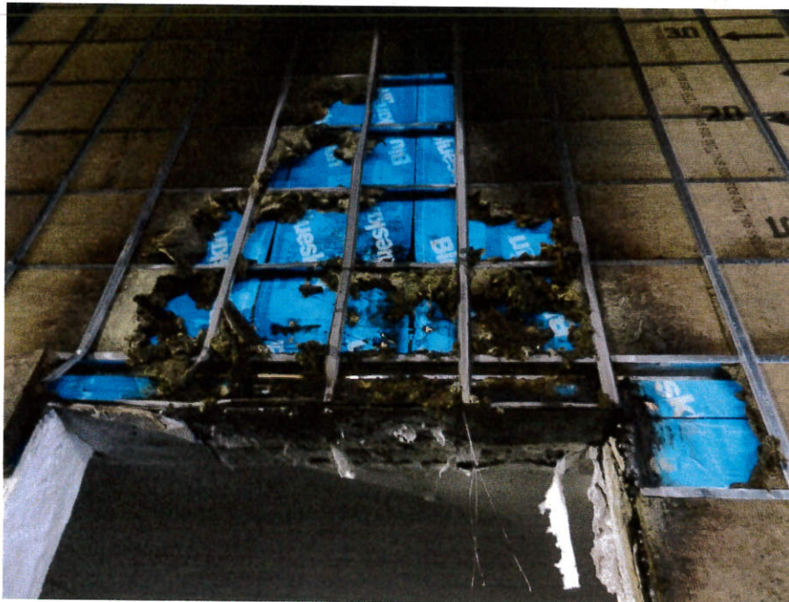
Figure 18. Insulation partially removed (showing water resistant barrier over CLT panels) after fire exposure.
