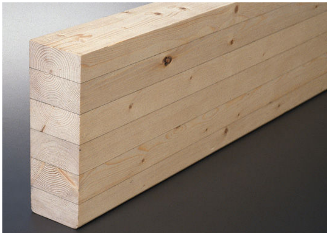
Figure 2.5 Glulam Member (Source: Figure 31L, section 4.1, FPI/TWBC)
