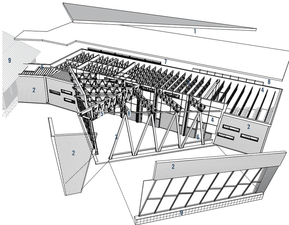
1. roof deck – constructed of vertical laminated SPF 2 x 4's
