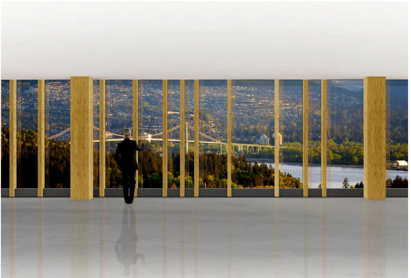
Interior perspective illustrating a glulam curtain wall
