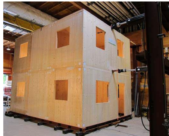
2 Storey CLT Structure Testing FPInnovations
