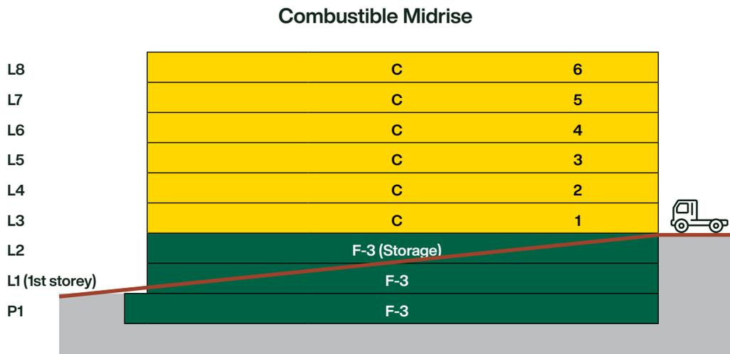
Figure 1. Building height addressed by alternative solution for allowing combustible construction (yellow) on a sloping site.
