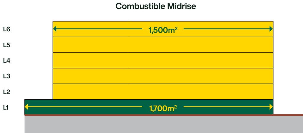
Figure 2. Excess building area addressed by alternative solution for allowing combustible construction (yellow).
