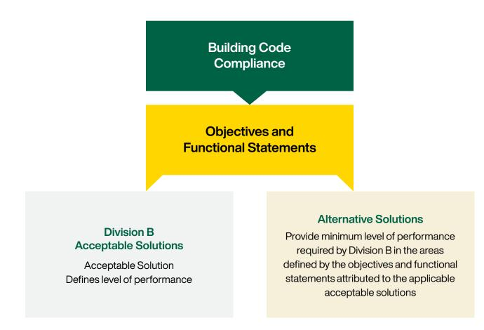
Acceptable solutions generally anticipate typical building situations that are common, with limited complications. The alternative solution path is an option for other situations, where acceptable solutions may not be appropriate, to enable flexibility in building construction. It provides design teams the ability to employ different design or construction methods that may differ from the prescriptive options envisioned by the building code.
