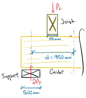
$A_b = 500 \text{ mm x } 215 \text{ mm} = 107500 \text{ mm}^2$
