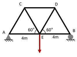
Dead load = 12 kN Live Load = 5 kN
