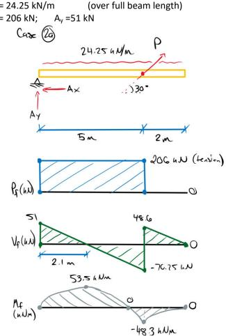
$P_f = 206 \text{ kN (tension)}$
