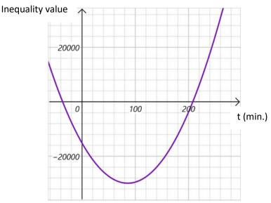
From this, we can see this inequality is satisfied for  $0 \le t \le ^2200$  min. which is within the relevant range for the FRR values calculated previously. Therefore, we must use the upper limit of the  $A_b$ ' calculation for the bearing resistance.
