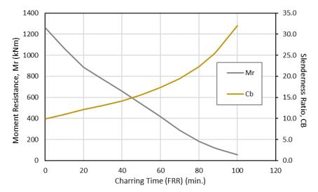
Here we can see that the critical FRR is around 88 minutes where the factored moment equals the remaining moment resistance. The slenderness ratio,  $C_b$  does not exceed the limit of 50 within this period and therefore does not govern the failure.
