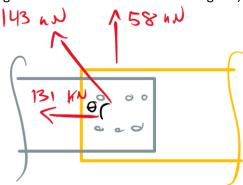
Therefore, the connection must be design for the governing individual loads above as well as both interactions for different  $\theta$  values (see **12.4.4.2 a-d**).
