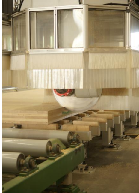
CNC machine to cut to size, make opening, fastener hole, etc
