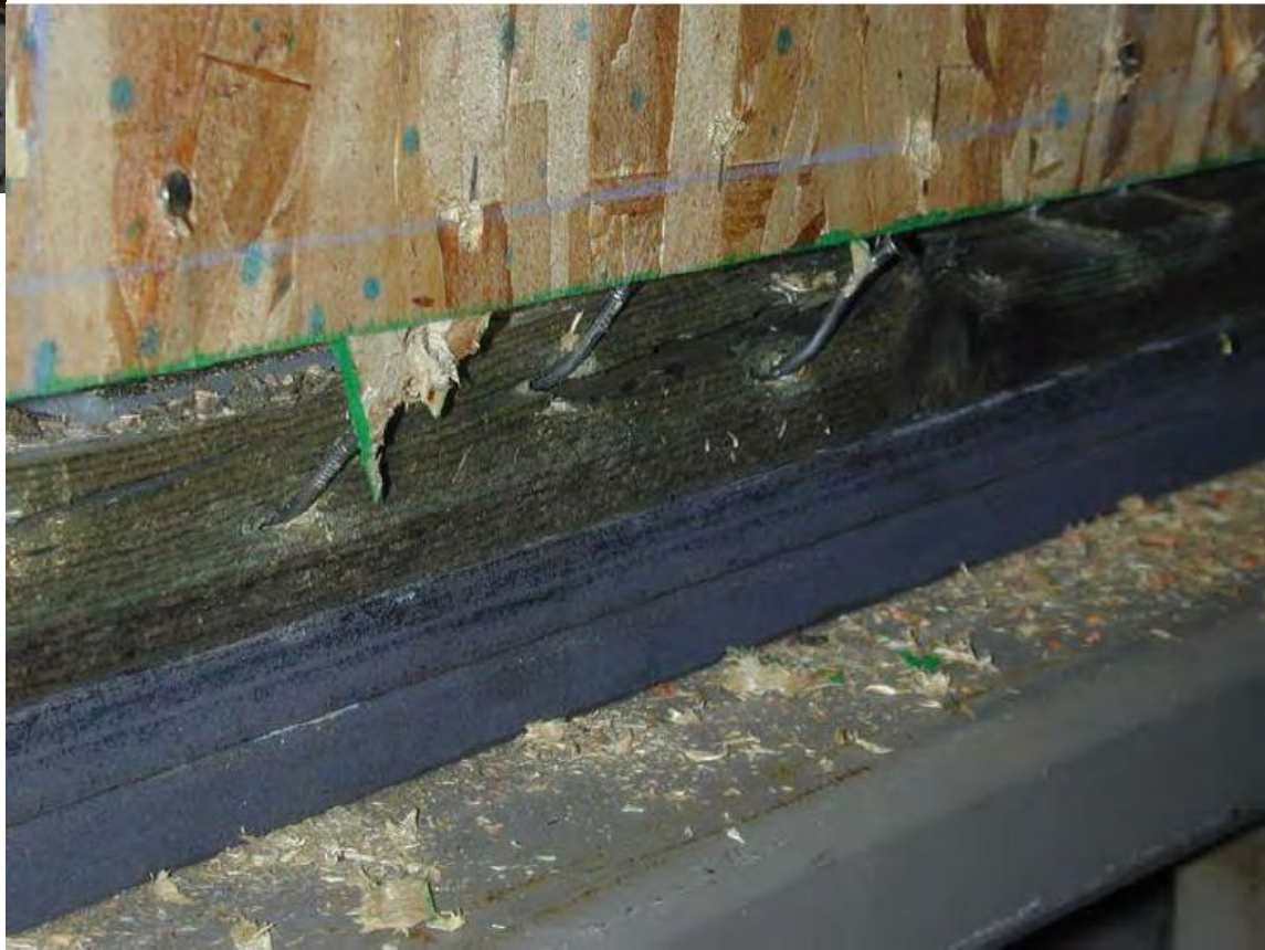
Nail bending/ripping through sheathing
