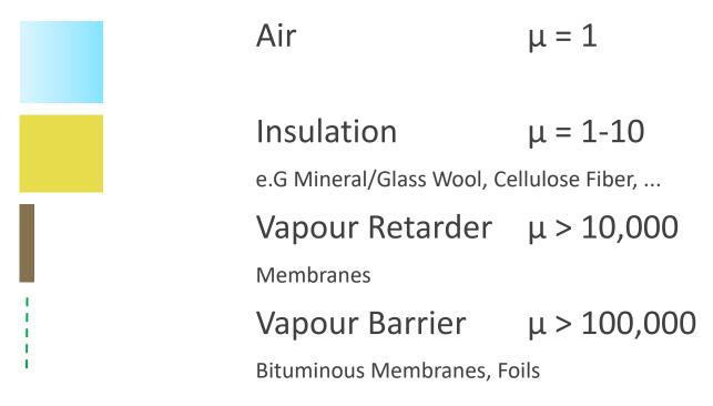
μ is the specific Vapour Diffusion Resistance of a specific material
