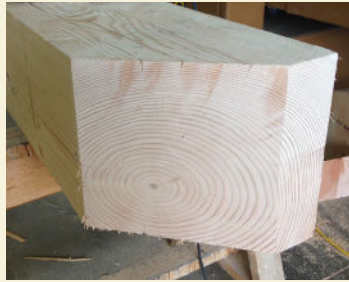
Solid-sawn mass timber
