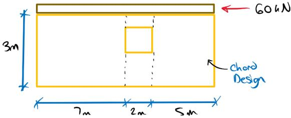
Assuming the wall stiffness is proportional to length we get the following factored shear force for the 5 m long wall.
