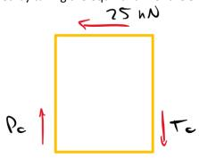
$$\Sigma M_p = 0 = -T_c(5 \text{ m}) + (25 \text{ kN})(3 \text{ m})$$
