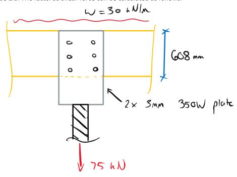
$$V_f = wL/2 + P_f/2 = (30 \text{ kN/m})(5 \text{ m})/2 + (75 \text{ kN})/2 = 112.5 \text{ kN}$$
