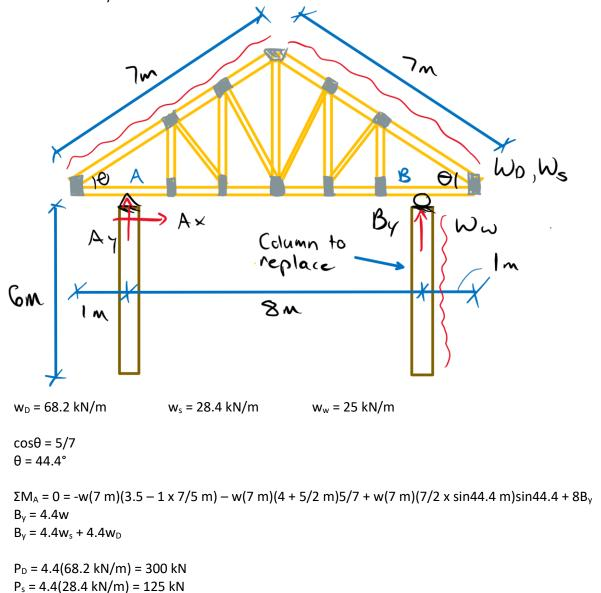
The column is in combined compression + bending, therefore we must identify the possible governing load cases.
