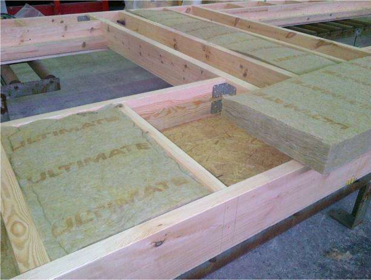
External Wall Element, Timber Frame, Glas Fiber Insulation, Off site production
